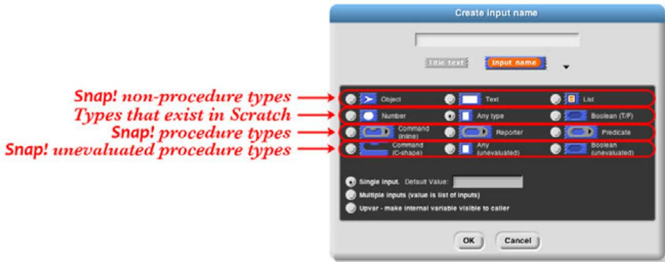
The second row of input types contains the ones found in Scratch: Number, Any, and Boolean. (The reason these are in the second row rather than the first will become clear when we look at the column arrangement.) The first row contains the new **Snap!** types other than procedures: Object, Text, and List. The last two rows are the types related to procedures, discussed more fully in section VI below.
